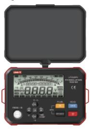
UT503PV has the function of measuring photovoltaic live insulation resistance (it can measure photovoltaic insulation resistance without power outage/short circuit of photovoltaic solar panels or at night, the maximum DC 1000V), ordinary insulation resistance function (non-live), AC and DC voltage automatic recognition measurement, stepping voltage, Bluetooth transmission, automatic discharge, high voltage live warning, remote control test pen operation test and other functions.
